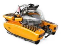
Tried and true, the *Triton 3300/3* is extremely versatile and thus a perfect choice for Esquel. Suited for both personal and scientific expeditions, this sub operates with a pilot and two passengers. It can travel to depths of 1000 meters (3,300 feet) in safety and comfort. It is the ideal vehicle for wreck diving and for viewing the magic of the underwater world. It was aboard a *Triton 3300/3* that man had his first underwater encounter with a giant squid! More adventures await.
